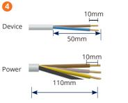
Cut the power and device cables to length.
